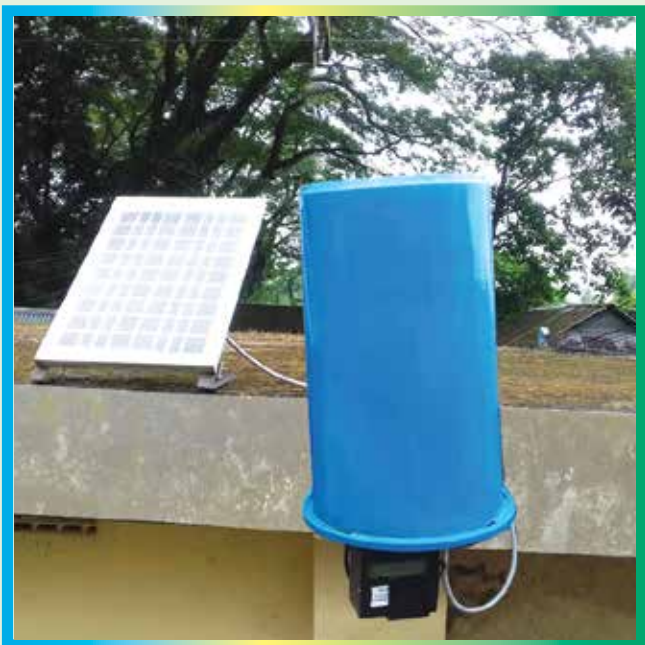
Figure 2: Automatic rain gauge
