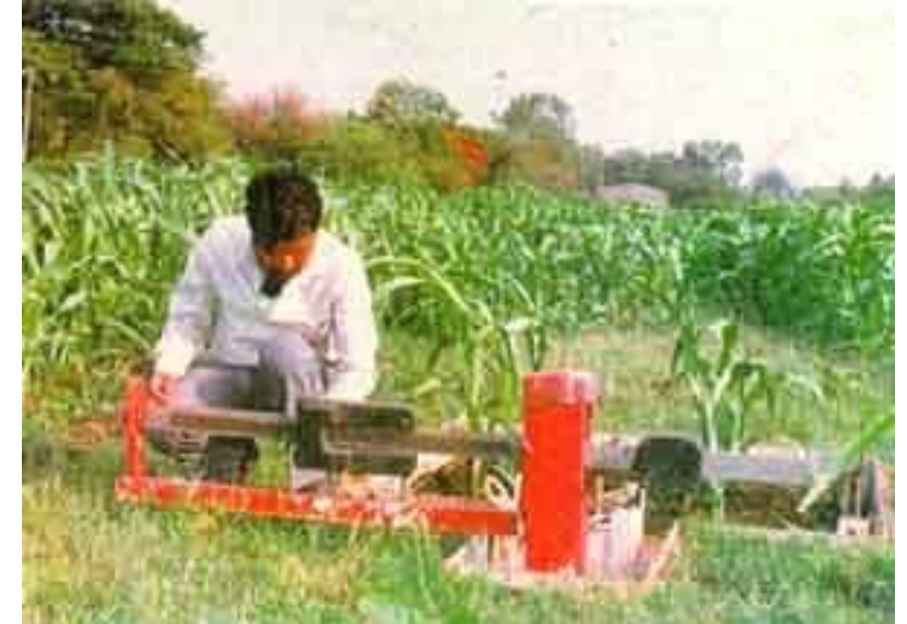
Evapotranspiration measurements by Gravimetric/volumetric lysimeters installed in crop environment
